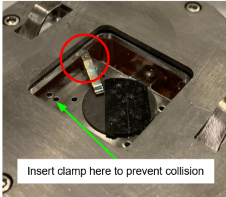
Figure 29. If the sample or sample clamps collide with the cover as shown in red, this may prevent evacuation and resealing. Either push down the clamp fully, or use a different hole to insert the clamp, as shown in green.
