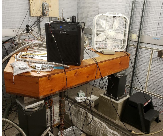
Figure 3.1. Calibrating the harmonic response of the STM with a speaker.
