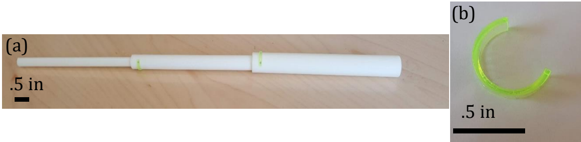
Figure 9: (a) 3_D Printed Prototype, extended with light green acrylic springs, (b) Zoom in on the acrylic springs
