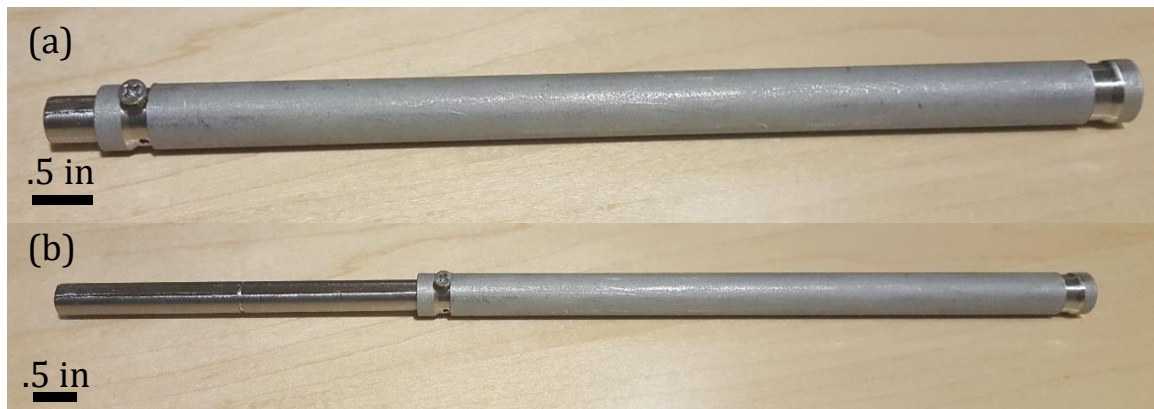
Figure 10: Stainless-steel 304 prototype (a) Retracted (b) Extended
