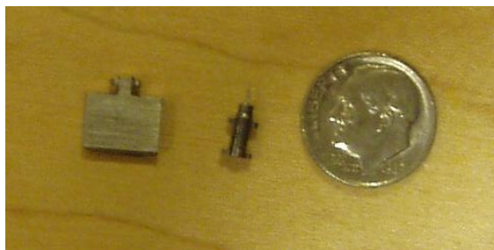
Figure 2.5: From left: the sample tray, on which the sample is mounted, an STM tip in its holder, and a dime. These are the actual objects that we grab out of the STM with a 6 foot long manipulator and bring to room temperature (not the dime).
